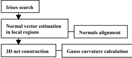
**Figure 1:** The algorithm of the image characteristics extraction.
